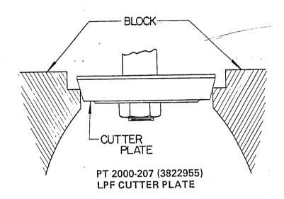
NOTE: LPF MACHINING REQUIRES THE USE OF(2) PT 2000-109 CUTTER BITS AND PT 2000-199 SPACER BLOCK.
