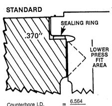
Counterbore I.D.  $= \frac{6.564}{6.570}$ Liner Flange O.D.  $= \frac{6.566}{6.564}$ Fit: .002" Press to .006" Clearance
