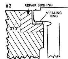
Repair Bushings PT-8000's Plus Seven O.S.'s Boring Dimensions: Standard Diameter: 6.750", Depth .600"
