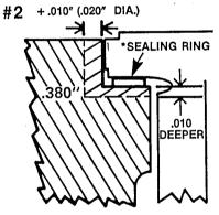
(1982) Machine Block for .020" O.S. Flange Liner
